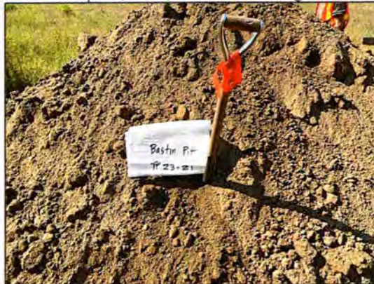
Test Pit 23-21 Spoil (High fines sand 5.5-6.0m)
