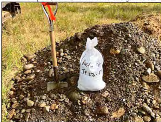
Test Pit 23-17 Spoil (Clean, coarse sand and gravel 0.2-5.5m)
