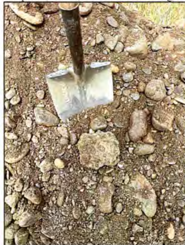
Test Pit 23-14 Spoil (Minor clay lumps at approximately 3.0m)
