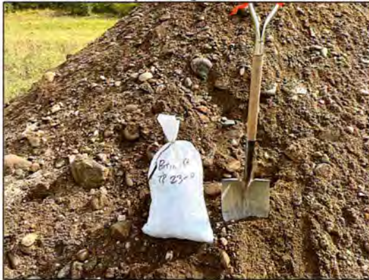
Test Pit 23-11 Spoil (Clean, coarse sand and gravel 1.4-4.0m)
