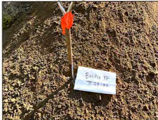
Test Pit 23-22 Spoil (High fines sand 1.8-6.0m)
