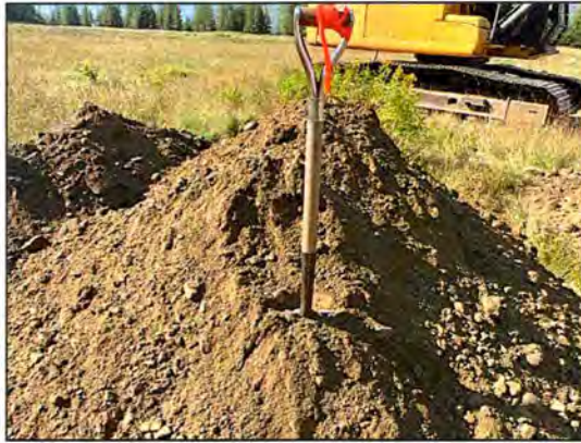
Test Pit 23-09 Spoil (High fines sand 2.8-6.0m)
