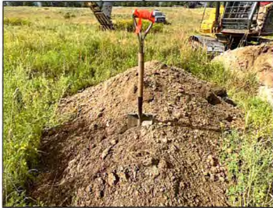
Test Pit 23-10 Spoil (High fines sand 0.1-5.0m)
