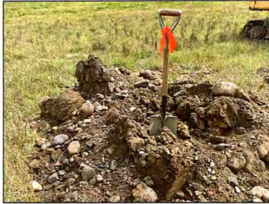
Test Pit 23-12 Spoil (Clay mixed with gravel 4.0-5.5m)
