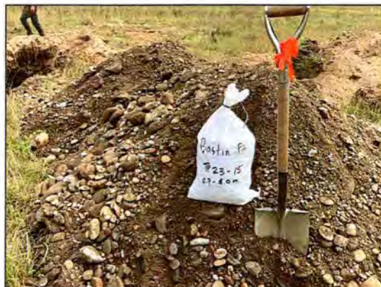
Test Pit 23-15 Spoil (Clean coarse sand and gravel 0.7-6.0m)
