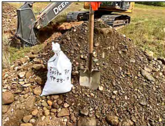
Test Pit 23-13 Spoil (Clean, coarse sand and gravel 0.1-5.5m)
