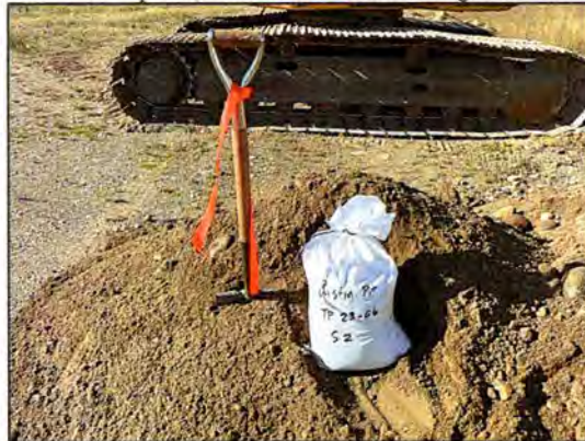
Test Pit 23-06 Spoil (High fines sand 4.2-5.4m)
