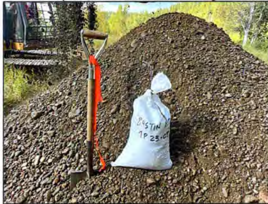
Test Pit 23-05 Spoil (Clean, coarse sand and gravel 2.0-4.5m)
