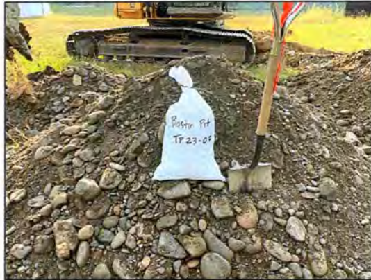
Test Pit 23-07 Spoil (Clean, coarse sand and gravel 0.5-5.0m)
