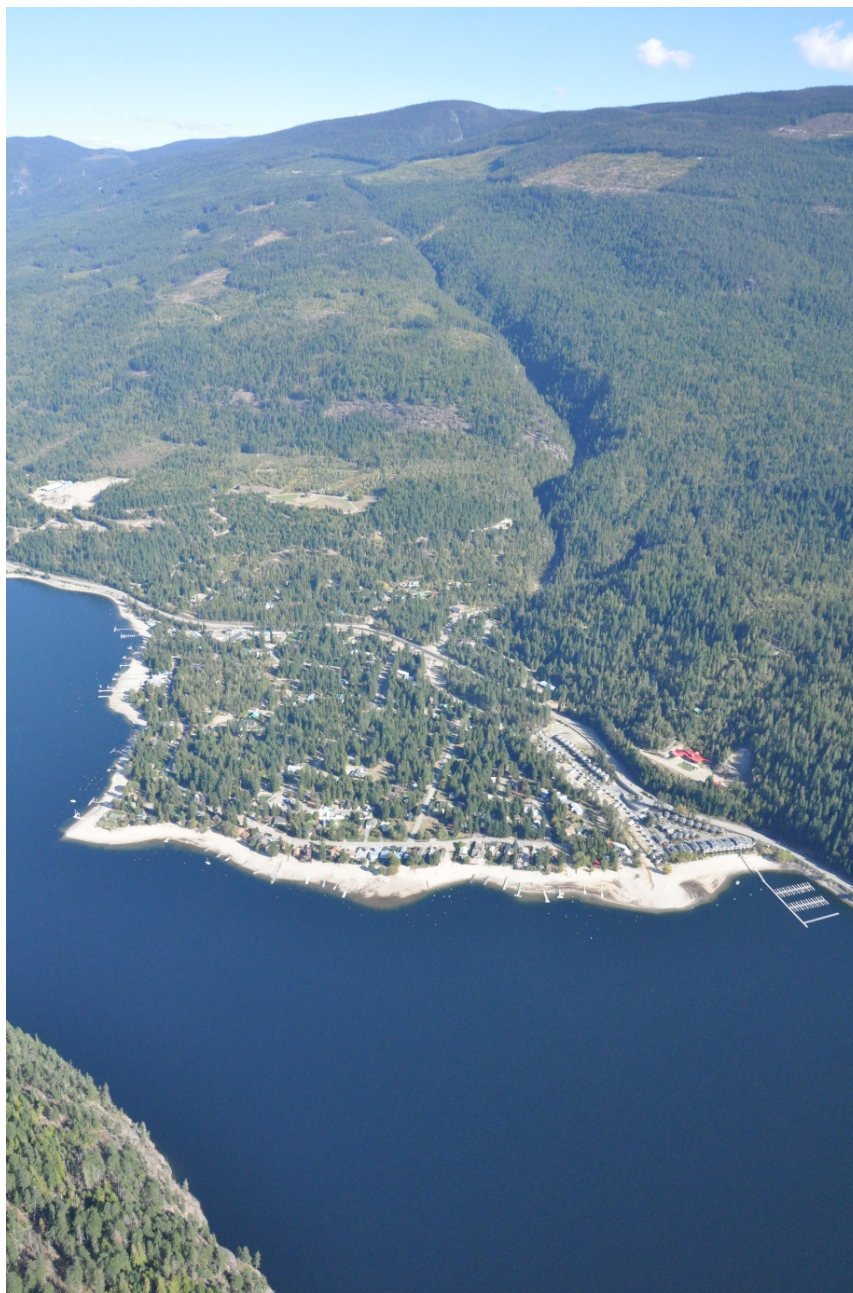
Photograph D-1. A typical steep creek watershed and fan (Hummingbird Creek) in the Thompson River Watershed, located near Sicamous. Photo: BGC taken on October 4, 2012.
