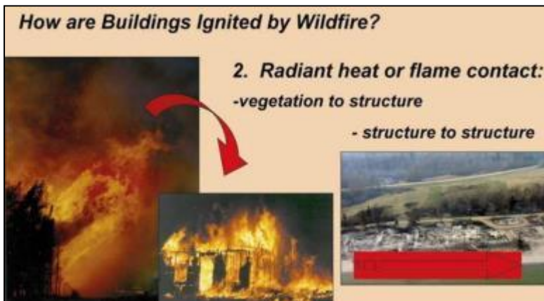
Figure 8. Radiant heat and flame contact allow fire to spread from vegetation to structure or from structure to structure.
