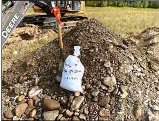
Test Pit 23-16 Spoil (Clean, coarse sand and gravel 0.2-5.5m)
