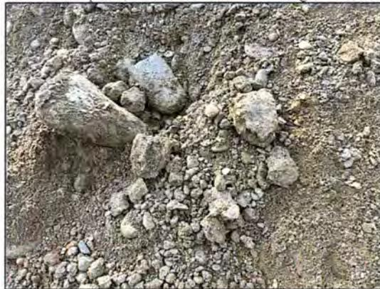
Test Pit 23-07 Spoil (Silt lumps mixed with gravel 5.0-6.0m)
