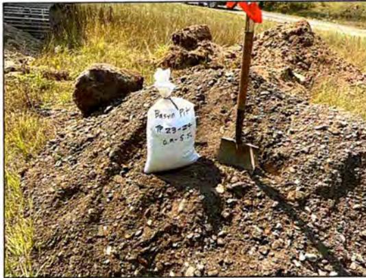
Test Pit 23-24 Spoil (Clean, coarse sand and gravel 0.9-5.5m)
