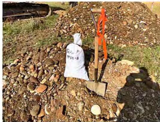
Test Pit 23-08 Spoil (Clean, coarse sand and gravel 0.1-4.6m)
