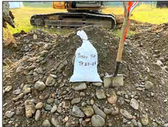
Test Pit 23-07 Spoil (Clean, coarse sand and gravel 0.5-5.0m)
