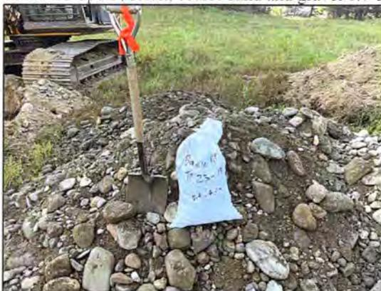
Test Pit 23-19 Spoil (Clean, coarse sand and gravel 0.4-5.0m)
