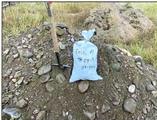
Test Pit 23-18 Spoil (Clean, coarse sand and gravel 0.7-5.0m)
