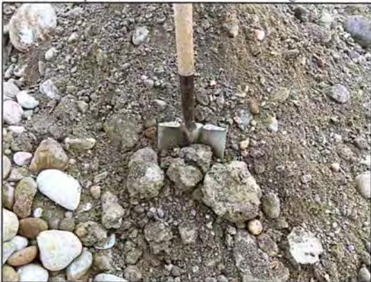
Test Pit 23-19 Spoil (Silt and clay mixed with gravel 5.0-5.5m)
