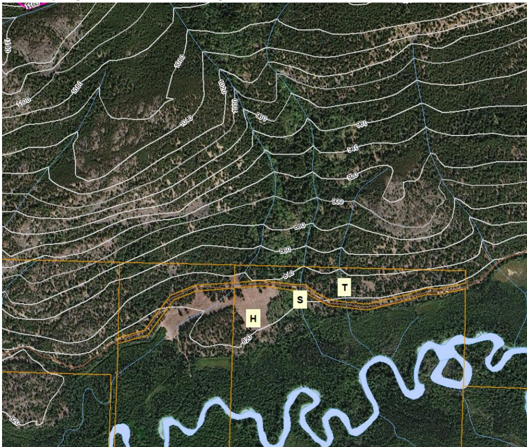
Figure 3. Approximate locations of the proposed septic and 45,000L storage tank, “S” and “T”, respectively, in relation to mapped streams (blue lines) from the Fresh Water Atlas spatial layer. “H” depicts the approximate heli pad location. Orange lines are district lot lines, white lines show elevation contours.
