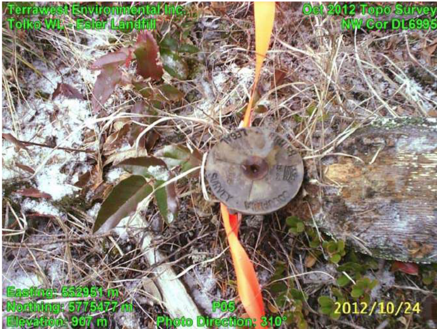
Photo 10. Legal survey corner pin to the Site.
