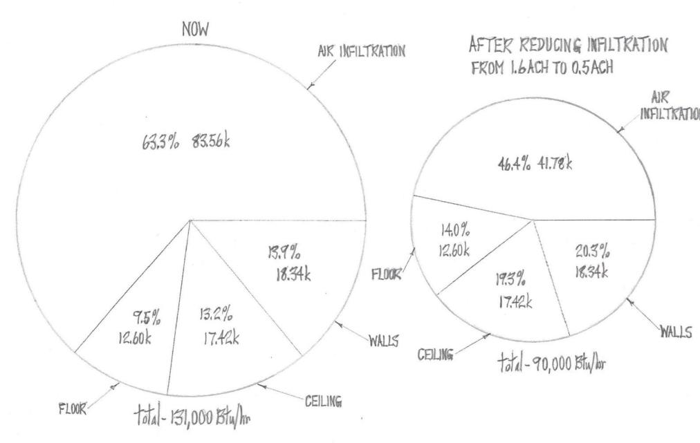
HORSEFLY COMMUNITY HALL heating load calculated for 21°C interior and -40°C exterior.
