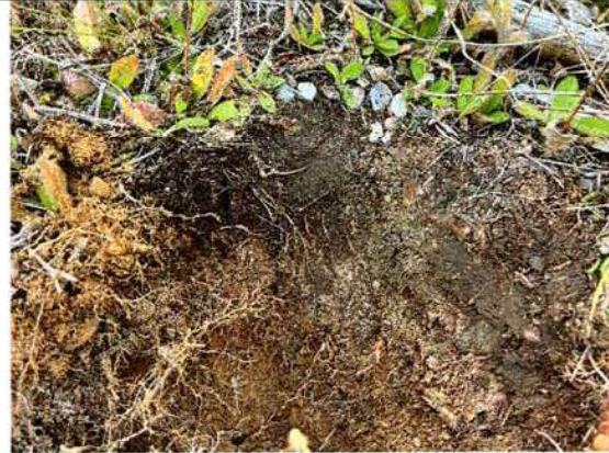
Photo 6: Top 30m of SS3 test pit facing east. Topsoil to 6cm sand with silt below, stones found throughout the soil profile with cobbles beginning around 90cm. Light brown, dry, loose.
