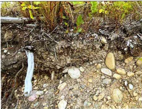
Photo 11: Representative soil profile where mining has occurred adjacent to the eastern disturbed area. About 5cm of topsoil is followed by about 15cm of B-Horizon. Topsoil and B-Horizon were consistent with the rest of Site. C Horizon was orange/ grey and was present from 15cm to about 200cm. Stones are found throughout the profile with cobbles beginning at about 20cm in depth.
